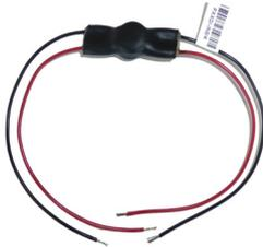
Supervised input kits are used with all inputs in the smoke control system. These kits protect the input and detect any trouble with the wiring (ground fault, short wire, etc.).
