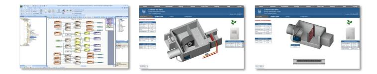
Distech Controls provides EC-Net<sup>AX</sup> wizards and EC-*gfx*Program, graphical programming interface, for the configuration and custom programming of our BACnet<sup>®</sup> and LONWORKS<sup>®</sup> controllers. These tools significantly improve efficiency of the engineering and programming processes in the EC-Net<sup>AX™</sup> solution.
